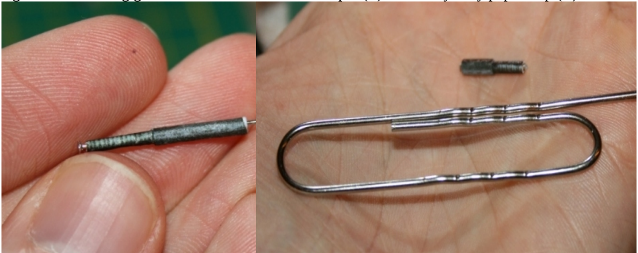
Figure 169: Landing gear strut construction around a pin (L) and heavy-duty paper-clip (R).
